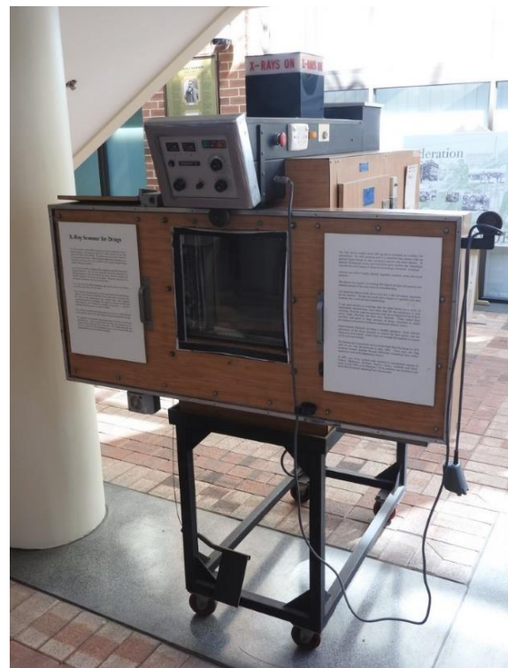
X-Ray Scanner for Drugs Developed after a number of Prototypes, by Customs Officer Leon Tate in 1976. By the late 1970's the machines were installed at Major Postal Control Centers around Australia
